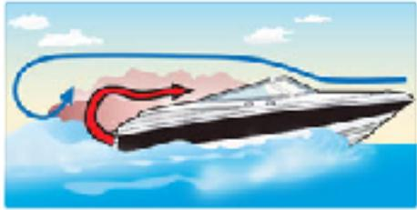
**Teak Surfing** or dragging or water skiing within 20 feet of a moving vessel can be fatal. If persons are using a swim platform or are close to the stern, all gasoline-powered generators with transom exhaust ports must be off.
